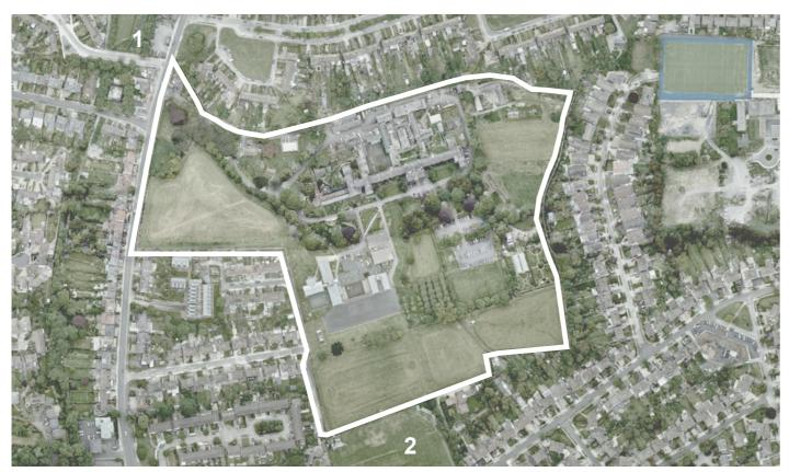
**Figure 46 -** Site Plan highlighting boundary wall in white. To increase site permeability and reduce the imposing character of the wall sections will be removed or reduced.
